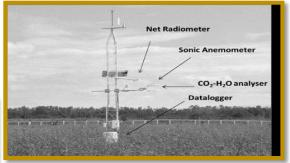
*Radiometers and Quantum Sensors:* Used to measure incoming and reflected solar radiation, including PAR, which is essential for assessing the energy available for photosynthesis.
